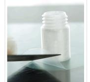
In cases of excess adhesion, it is recommended to wet print bed with a small amount of water slowly working it below the part. This should make part removal easier.
